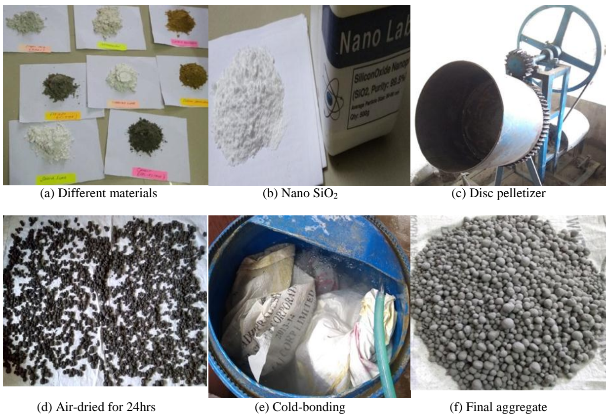
Figure 1 Manufacturing process of the artificial lightweight aggregates
