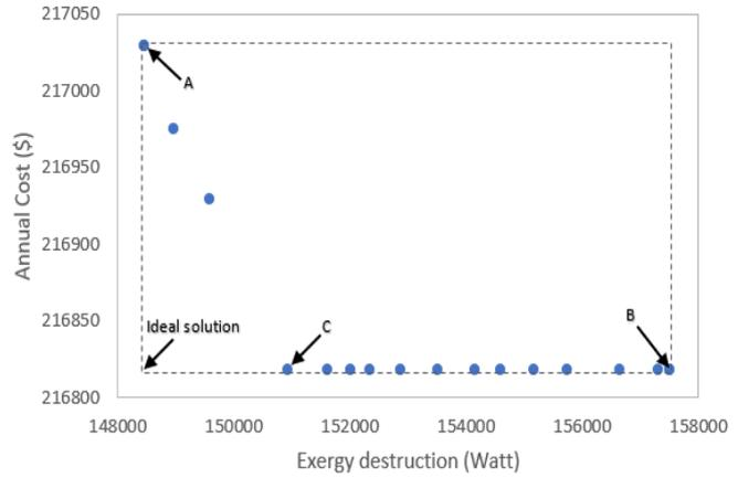
Figure 3 Result of multi-objective optimization for zeolite-water working pairs
