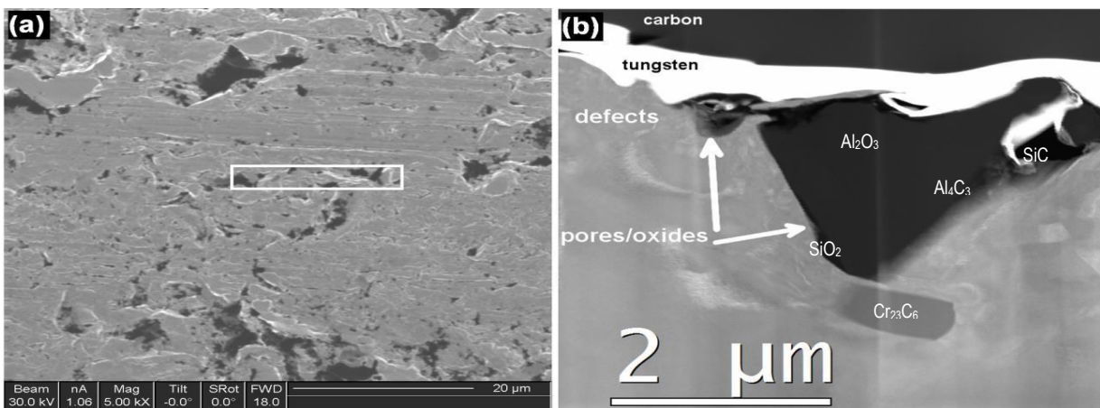
Figure 6 (a) FIB-SEI on surface of 73Fe24Cr2Si0.8Mn0.1Ni steel; (b) TEM image on depth of surface 3.5 \mu\text{m} of 73Fe24Cr2Si0.8Mn0.1 Ni steel
