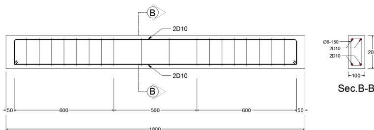
Figure 3 Beam with Double Reinforcement (SFRC-DR)
