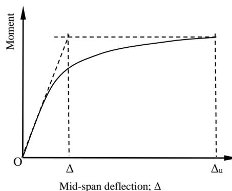
Figure 7 Ductility measurement
