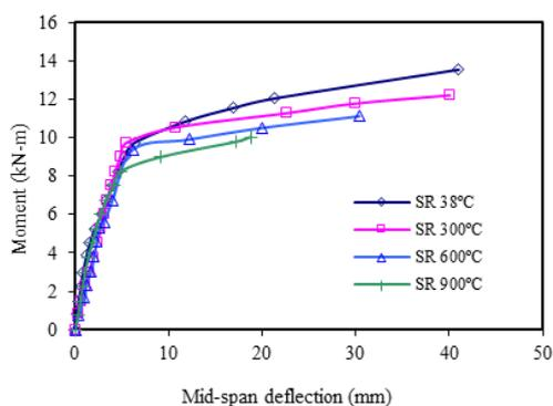
Figure 10 Moment versus mid-span deflection of the SFRC-SR specimens
