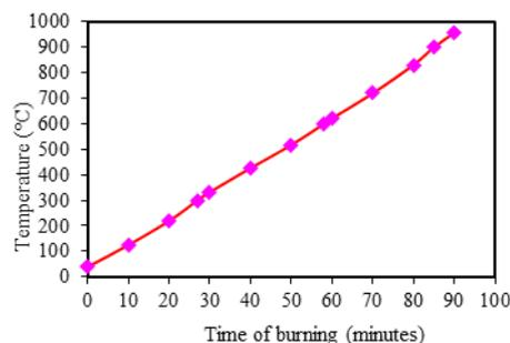
Figure 5 Relationship between time of combustion and temperature
