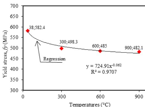
Figure 8 Average Yield Stress of Longitudinal Reinforcement at Elevated Temperatures
