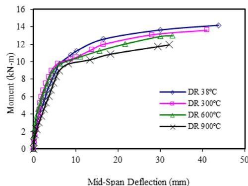
Figure 11 Moment versus mid-span deflection of the SFRC-DR specimens
