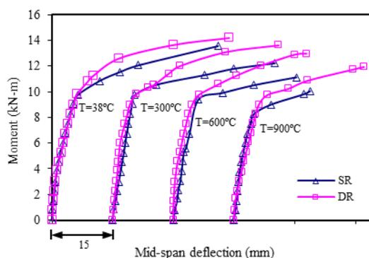
Figure 12 Comparison of SFRC beams with single and double reinforcement
