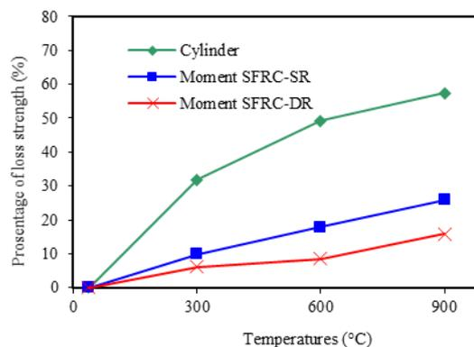
Figure 9 Loss strength of cylinder and beams
