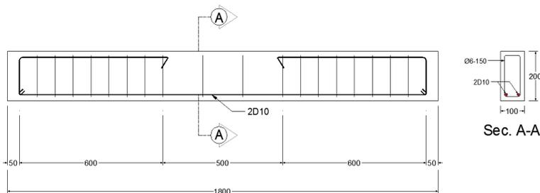
Figure 2 Beam with Single Reinforcement(SFRC-SR)
