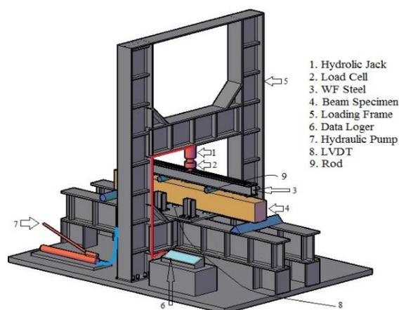
Figure 6 Testing scheme of the pure bending on the beam
