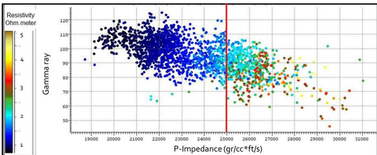
Figure 1 Cross-plot with P-impedance as the x-axis, gamma rays as the y-axis, and resistivity as color. P-impedance cutoff was defined at 25,000 gr/cc\*ft/s (red line)
