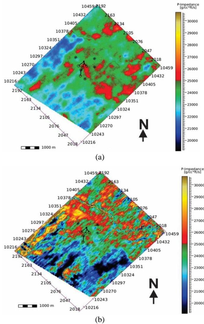
Figure 7 The P-impedance map along layer M, which was produced by: (a) geostatistical seismic inversion; and (b) deterministic seismic inversion
