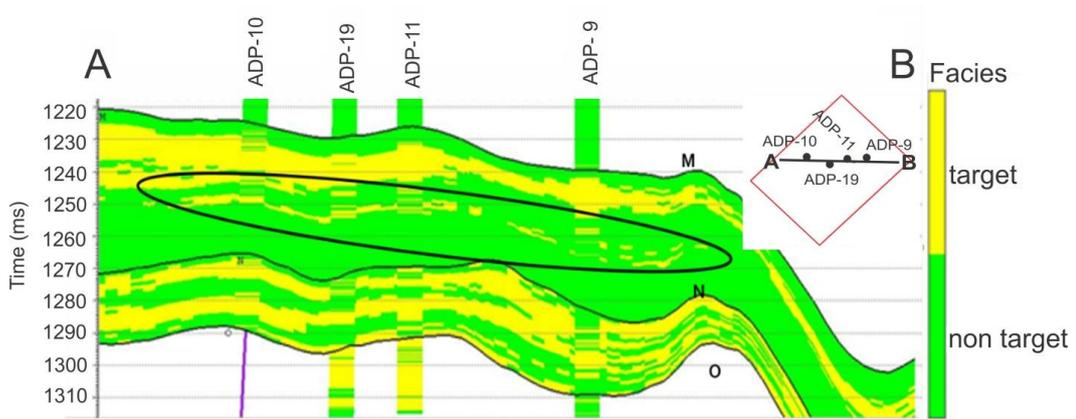
Figure 6 The discrete properties model for line AB. The black ellipse shows the thin reservoir.
