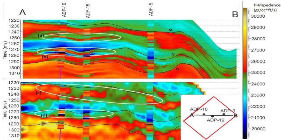
Figure 3 The comparison between the geostatistical seismic inversion result (top) and deterministic seismic inversion result (bottom) for line AB, where the inserted well log data are P-impedance. The ADP-09 well was not included in the inversion process, but it was used to verify the inversion result
