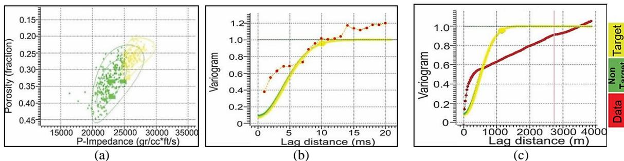
Figure 2 The statistical analysis for layer M that consists of: (a) the probability density function; (b) vertical variogram from porosity data; and (c) lateral variogram from P-impedance data (gr/cc\*ft/s). The red, green, and yellow colors indicate the experimental, non-target, and target variogram models, respectively
