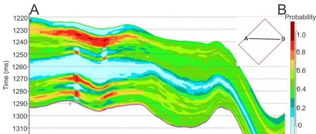
Figure 5 The probability model for line AB, which was produced based on 50 realizations. The black ellipse shows the target reservoir
