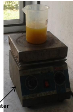
Figure 7 Oil sample on the magnetic stirrer
