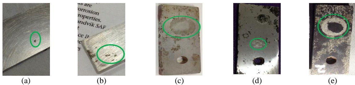
Figure 2 Visual observation of SAF 3207 HD after weight loss in 6% FeCl 3 with solution temperature of: (a) 60°C; (b) 65°C; (c) 70°C; (d) 80°C; and (e) 90°C for 72 hours
