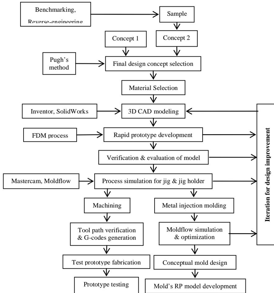
Figure 1 Flow chart of the prototype development process
