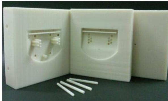
Figure 9 RP model of the conceptual mold design
