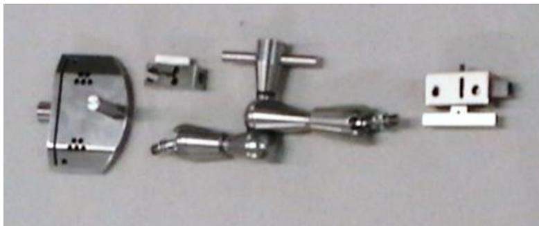
Figure 5 Jig and jig holder components
