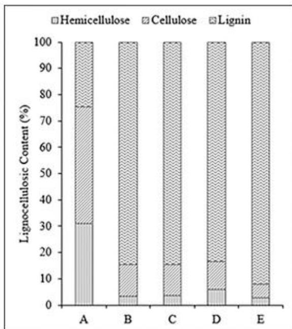
Figure 4 Lignocellulosic contents of raw and torrefied sugarcane bagasse at various torrefaction heating rates and hold times, (A) raw bagasse; (B) torrefied bagasse at 3°C/min, 0 minute; (C) at 6°C/min, 0 minute; (D) at 10°C/min, 0 minute; and (E) at 6°C/min, 15 minutes
