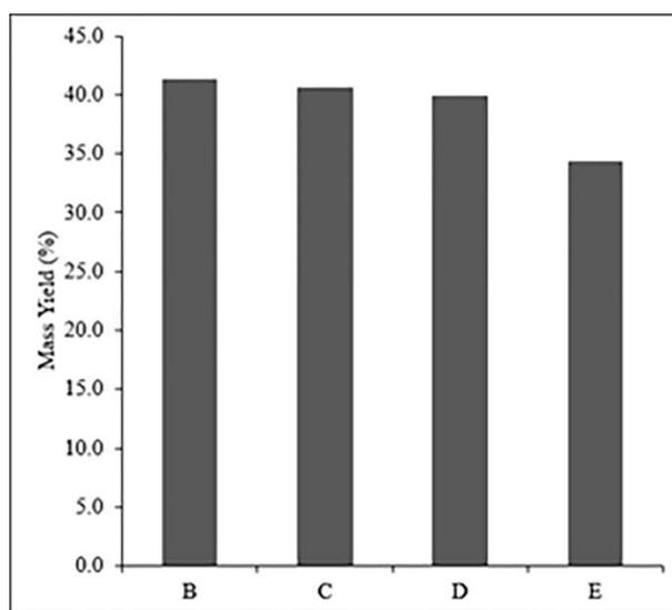
Figure 3 Mass yield distributions of torrefied sugarcane bagasse at various torrefaction heating rates and hold times, (B) at 3°C/min, 0 minute; (C) at 6°C/min, 0 minute; (D) at 10°C/min, 0 minute; and (E) at 6°C/min, 15 minutes, respectively
