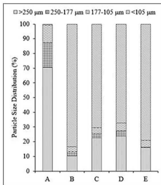
Figure 5 Particle size distributions of raw and torrefied sugarcane bagasse at various torrefaction heating rates and hold times. Symbols refer to Figure 4
