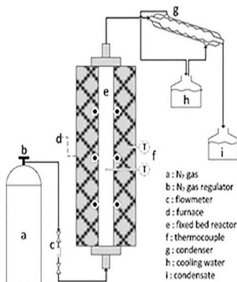
Figure 1 Experimental system of sugarcane bagasse torrefaction
