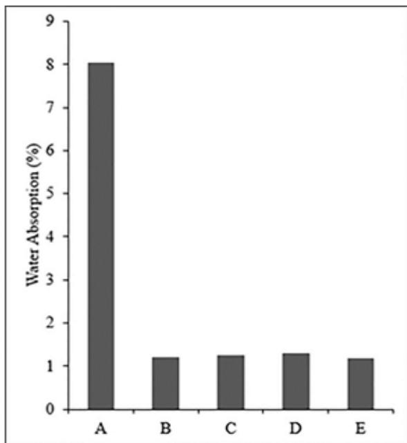
Figure 6 Water absorption of raw and torrefied sugarcane bagasse at various torrefaction heating rates and hold times. Symbols refer to Figure 4
