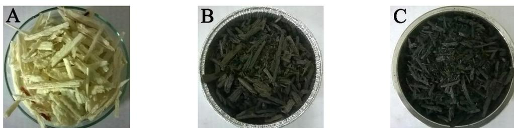
Figure 2 (A) Prepared raw sugarcane bagasse; (B) Torrefied sugarcane bagasse (char) at heating rate and hold time of  $6^{\circ}\text{C}/\text{min}$  and 0 minute, respectively; (C) Torrefied sugarcane bagasse at heating rate and hold time of  $6^{\circ}\text{C}/\text{min}$  and 15 minutes, respectively
