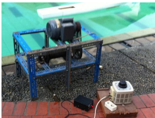
Figure 4 Motor used to pull the ship model
