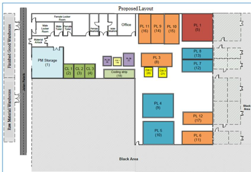
Figure 7 Proposed layout of Secondary Packaging Area
