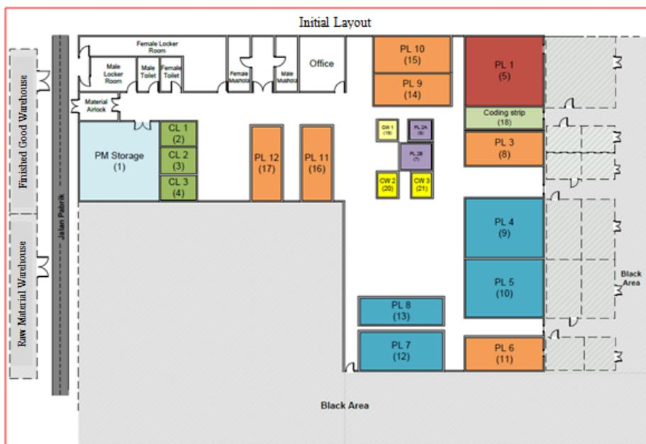
Figure 6 Initial layout of the Secondary Packaging Area
