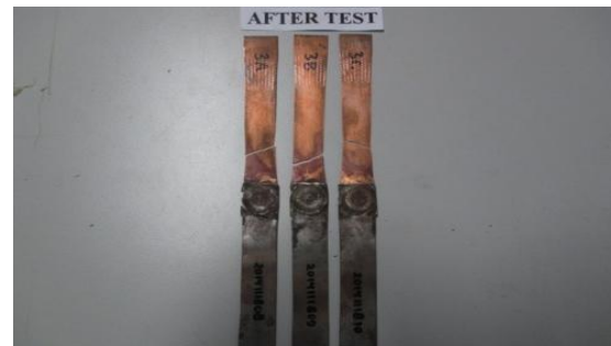
Figure 6 Sample after tensile test
