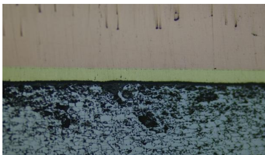
Figure 9 Microstructures of Dissimilar Metal Joining on Torch Brazing at 200×
