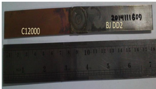
Figure 5 Joint specimen using Torch Brazing
