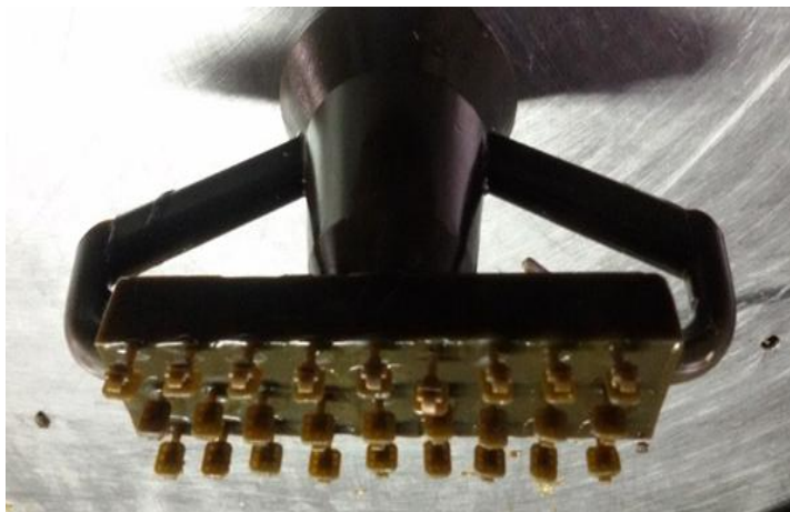
Figure 7 Tree configuration of wax in investment casting
