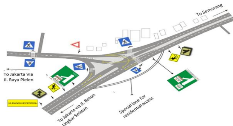
Figure 8 Proposed change of Gringsing Roundabout to a Y-junction and lay-out plan of road markings and signage
