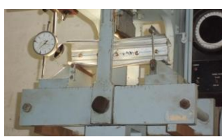
Figure 5 Flexural testing of cold-formed steel beams
