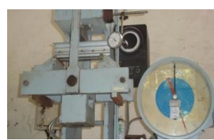
Figure 5 Flexural testing of cold-formed steel beams
