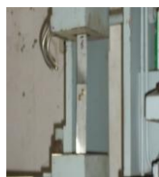
Figure 4 Axial testing of single lap joints (SLJs)
