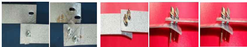
Figure 10 Axial joint failure of screw connection due axial loading
