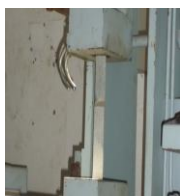
Figure 4 Axial testing of single lap joints (SLJs)
