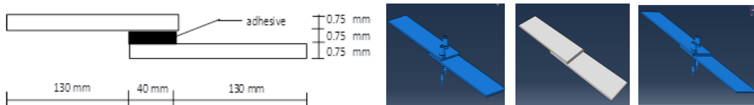
Figure 1 Single lap joint specimens of 42 mm width
