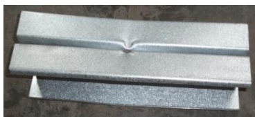
Figure 12 Flexural screw joint failure of cold-formed steel specimen
