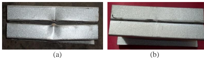
Figure 13 Combination joint's failure of flexural cold-formed steel; (a) screw and an epoxy resin adhesive, (b) screw and a polyester resin adhesive
