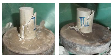
Figure 7 Adhesive failure of cylindrical an epoxy resin specimens
