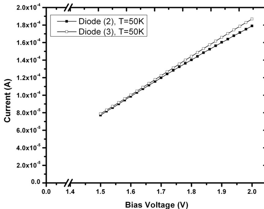
Figure 7 Linear I-V characteristics of diode (2) and diode (3) under a temperature of 50 K
