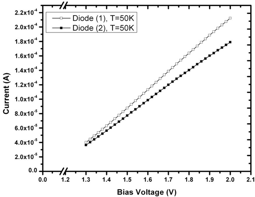
Figure 5 Linear I-V characteristics of diode (1) and diode (2) under the temperature of 50K
