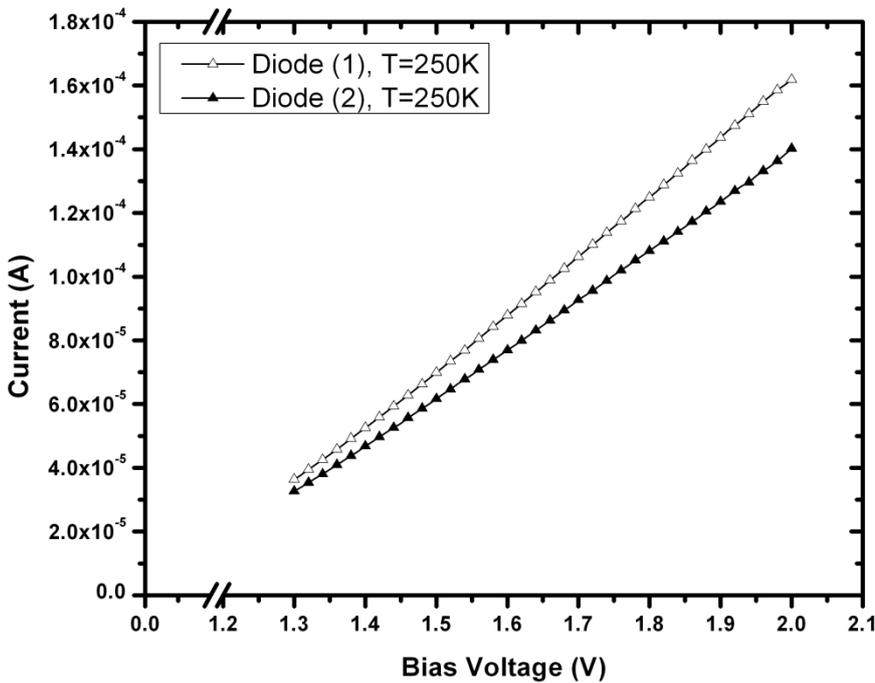
Figure 6 Linear I-V characteristics of diode (1) and diode (2) under temperature of 250 K
