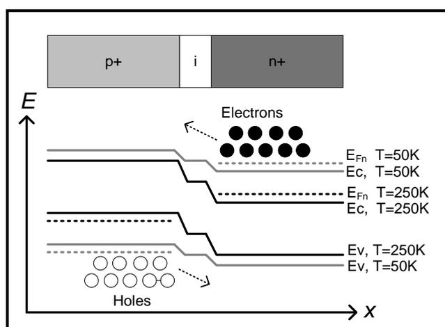
Figure 9 The energy band diagram of highly-doped nanoscale  $p-i-n$  diode
