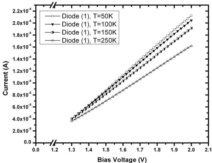
Figure 2 Linear I-V characteristics of diode (1) as a function of temperature
