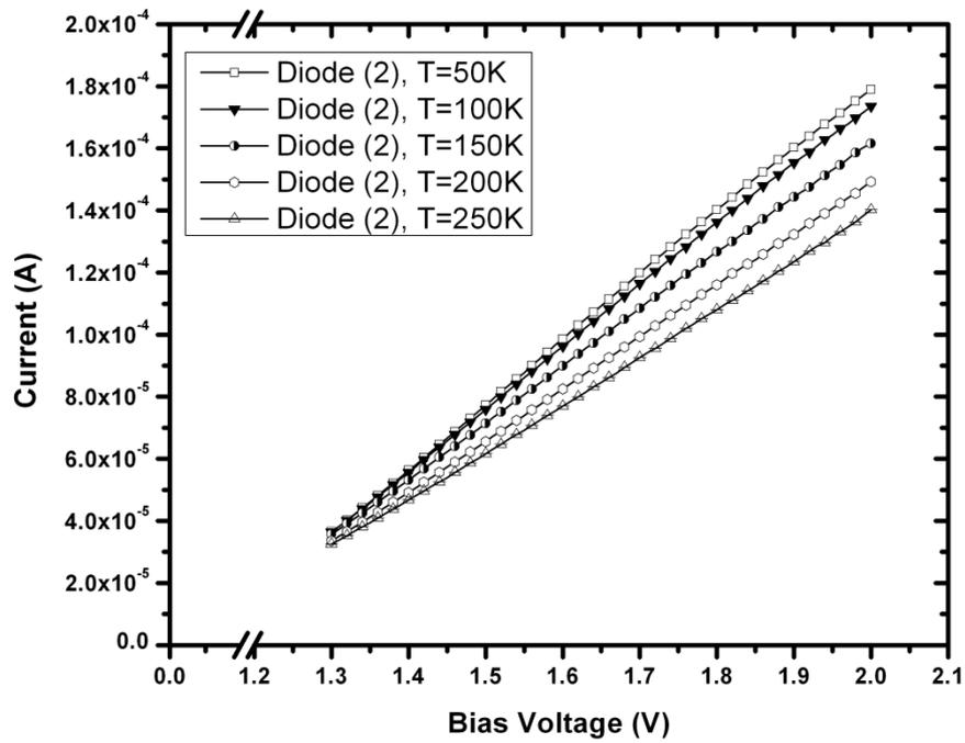
Figure 3 Linear I-V characteristics of diode (2) as a function of temperature
