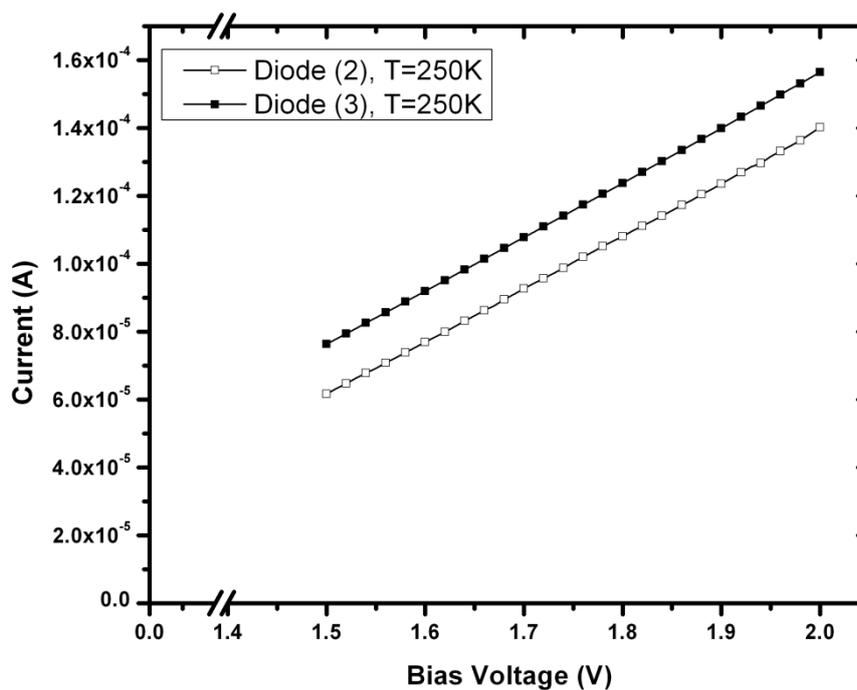
Figure 8 Linear I-V characteristics of diode (2) and diode (3) under a temperature of 250 K
