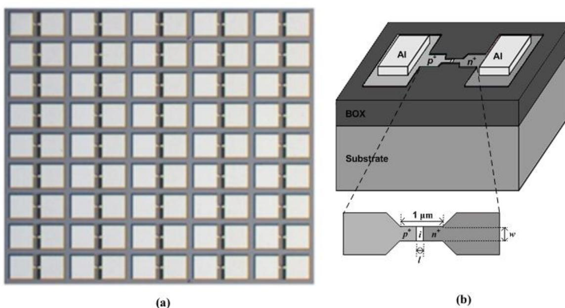
Figure 1 SOI  $p$ - $i$ - $n$  diode: a) photograph; b) structure
