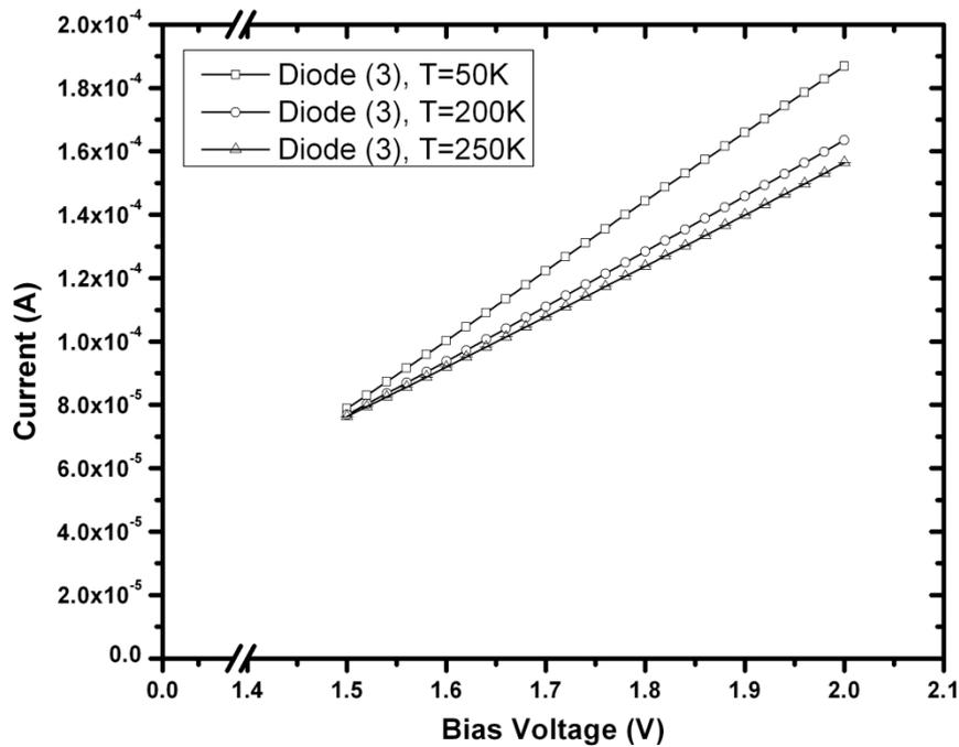
Figure 4 Linear I-V characteristics of diode (3) as a function of temperature
