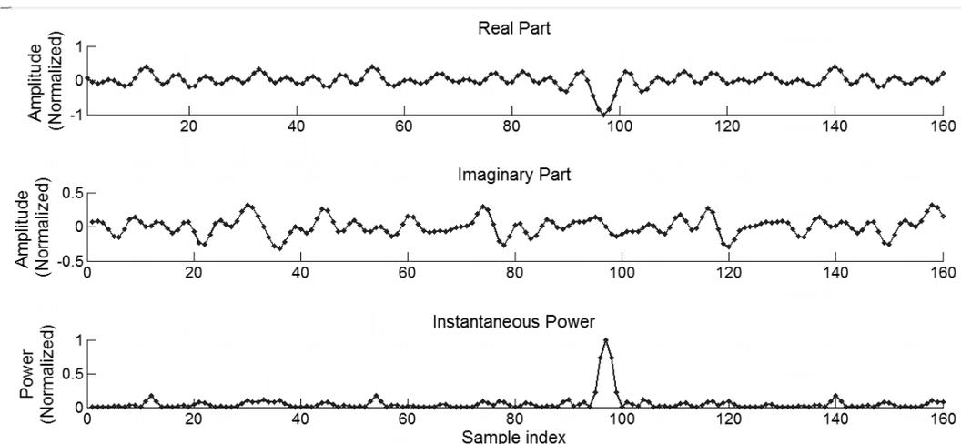
Figure 6 L-SIG signal that has maximum PAPR
