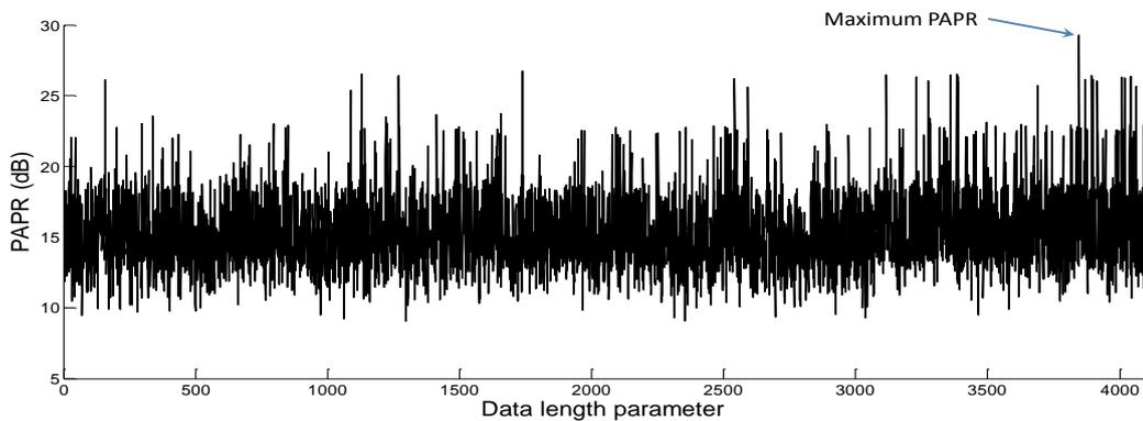
Figure 5 PAPR as a function of data length parameter for the L-SIG field
