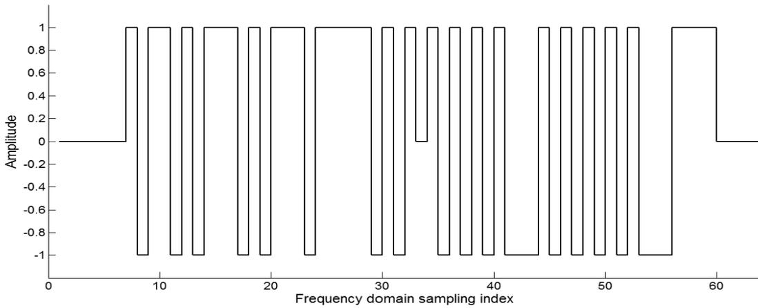
Figure 9 IFFT input of L-SIG signal
