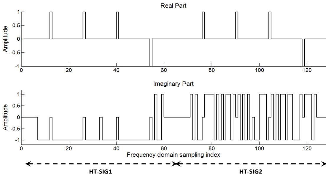
Figure 10 IFFT input of HT-SIG signal
