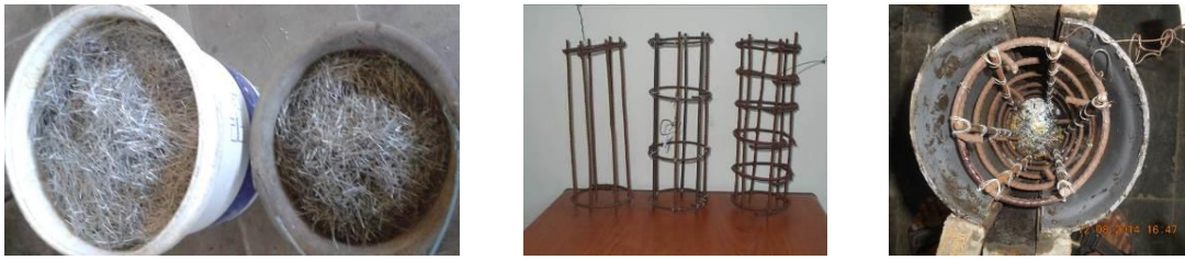
Figure 1 Steel fiber and reinforcement of specimens
