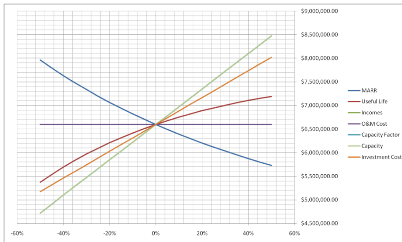
Figure 6 Spiderplot graph for sensitivity analysis, where X axis is percent based on normal value (%) and Y axis is present value (US$)
