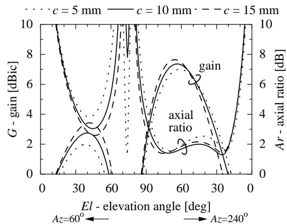
Figure 5 Gain and axial ratio versus elevation angle (patch #3 off)
