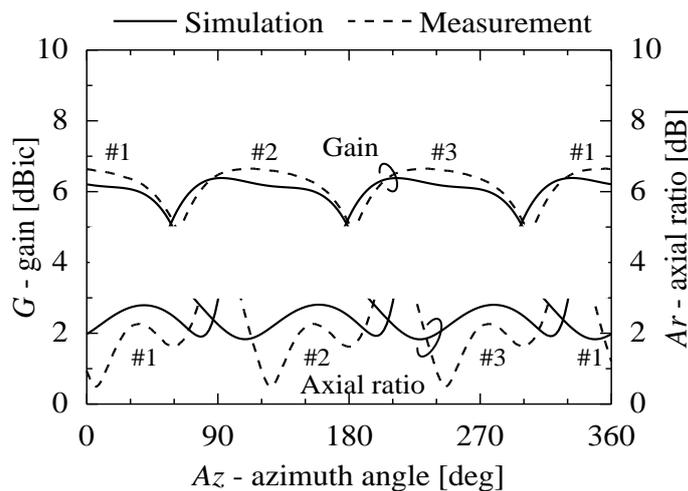
Figure 10 Switched beam characteristics in the conical-cut plane ( $El = 48^\circ$ )
