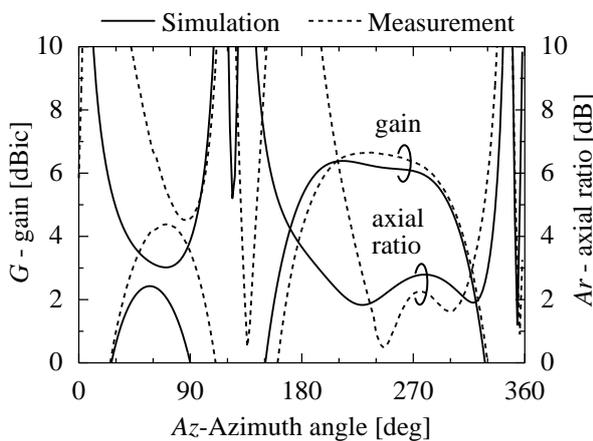
Figure 8 Radiation characteristics in a conical cut (patch #3 off,  $El = 48^\circ$ )
