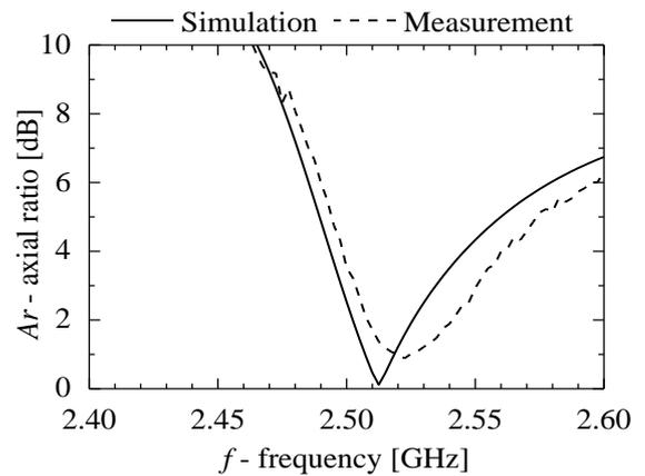
Figure 7 Axial ratio versus frequency
