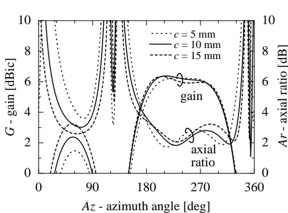
Figure 4 Gain and axial ratio versus azimuth angle (patch #3 off)
