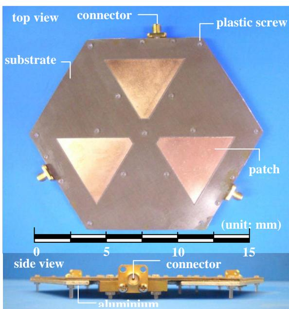
Figure 2 Fabricated antenna
