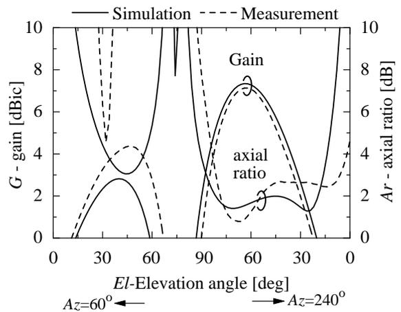
Figure 9 Radiation characteristics in an elevation cut (patch #3 off,  $El = 48^\circ$ )
