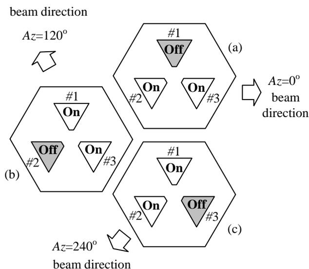
Figure 3 Switching mechanism of the developed antenna: (a) patch #1 off; (b) patch #2 off; (c) patch #3 off
