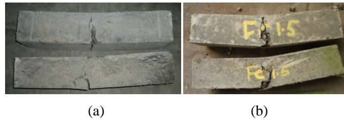
Figure 3 Failure pattern of specimen: (a) three point bending; (b) impact test
