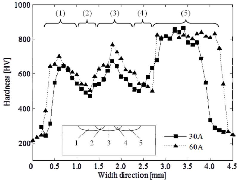
Figure 7 Hardness distribution of multiple passes with different arc currents
