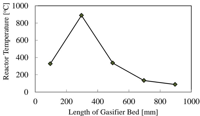
Figure 4 Typical temperature profile along gasifier bed
