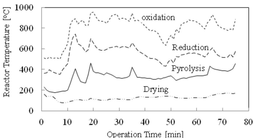
Figure 2 Dynamic temperature profile of the various gasification zones
