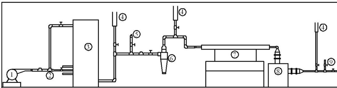
Figure 1 Schematic drawing of experimental setup: (1) air blower, (2) air distribution line, (3) downdraft gasifier, (4) gas flare points, (5) raw gas sampling point, (6) cyclone for gas cleaning, (7) cooling heat exchanger, (8) oil bath filter, (9) clean gas sampling point
