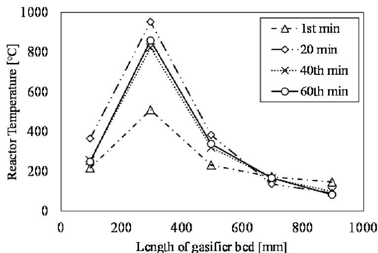
Figure 5 Variation of temperature profile along gasifier bed, at different operation time
