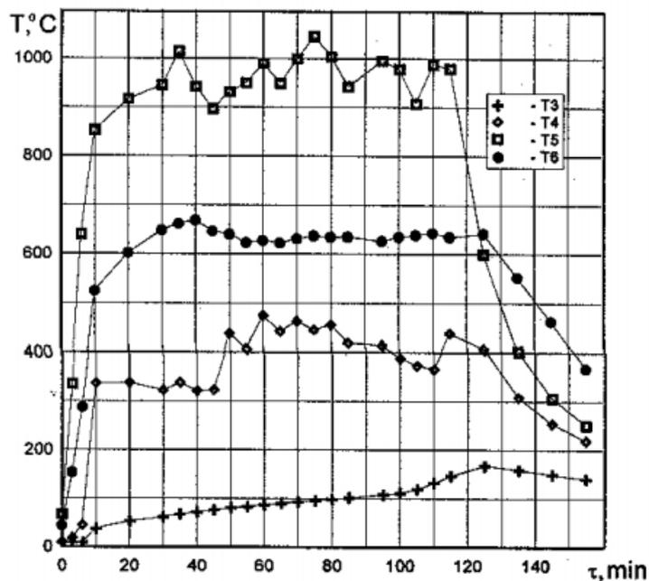
Figure 3 Dynamic temperature profile for downdraft gasification of wood (Borisov et al., 1998): T3 – drying zone, T4 – pyrolysis zone, T5 – Combustion zone, T6 – Reduction zone
