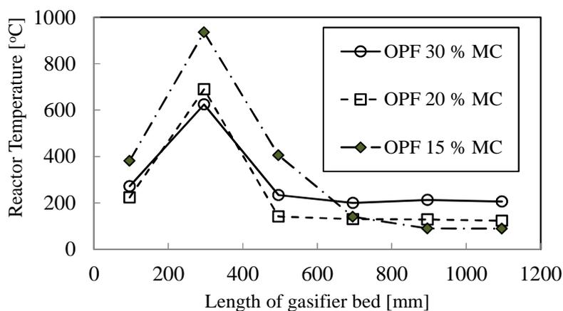
Figure 6 Variation of reactor temperature along the gasifier bed for different initial moisture content of OPF
