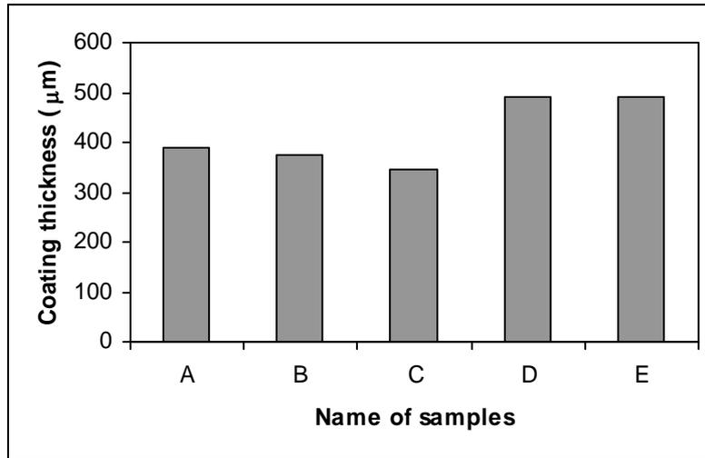
Figure 2 Variety of WC-Co coating thickness on samples with different surface roughness. Sample A: without grit blasting, and other samples with grit blasting with the pressure of: B: 0.1 MPa, C: 0.3 MPa, D: 0.4 MPa and E: 0.5 MPa
