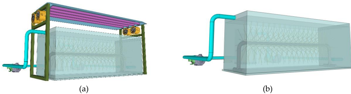
Figure 6. Reactor photocatalytic in (a) UV experimental setup, (b) Hypothetical design for sunlight photocatalytic reactor
