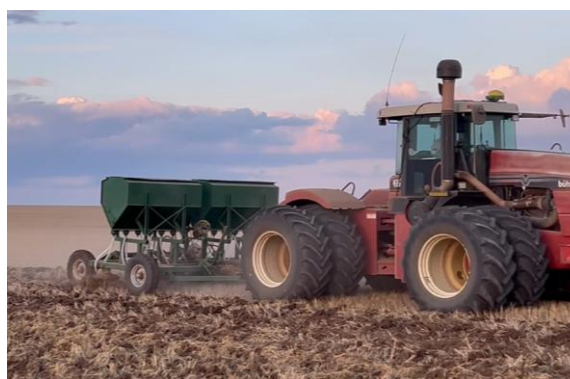
Figure S1 Photos from field tests of the deep loosener-fertilizer
