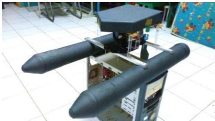
Figure 1 Proposed USV rocket with double hull
