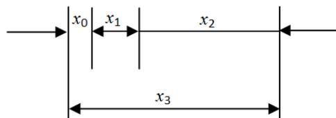
Figure 2 The dimension chain of the assembly
