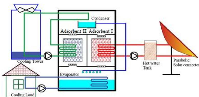
Figure 1 Schematic Diagram of a Two-bed Solar Adsorption Chiller
