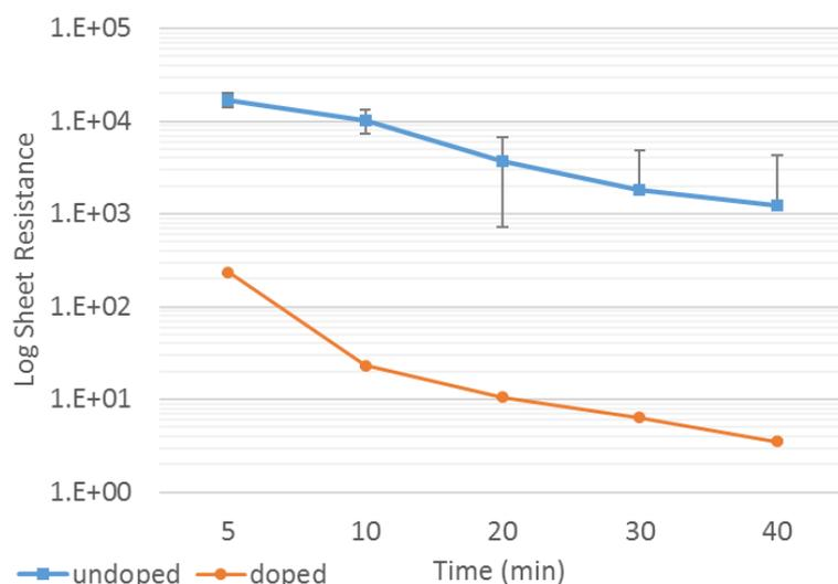
Figure 3 The electrical resistivity of the undoped and fluorine doped TCO glasses
