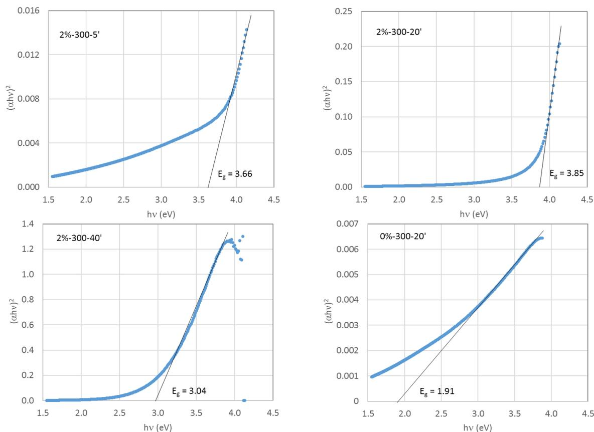
Figure 7 Optical band gap using Tauc equation
