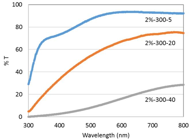
Figure 5 Optical transmittance of the fluorine doped samples with 5, 20, and 40 minute deposition times
