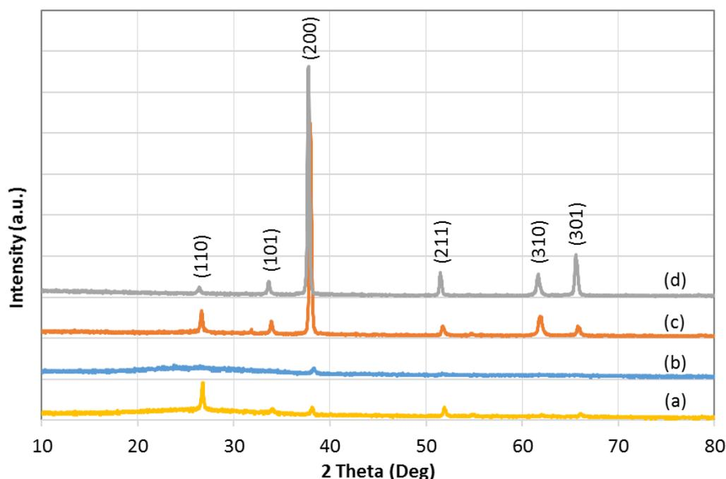
Figure 2 Diffractogram of TCO glasses under condition of: (a) undoped (0%-300-20'); (b) doped (2%-300-5'); (c) doped (2%-300-20'); (d) doped (2%-300-40')
