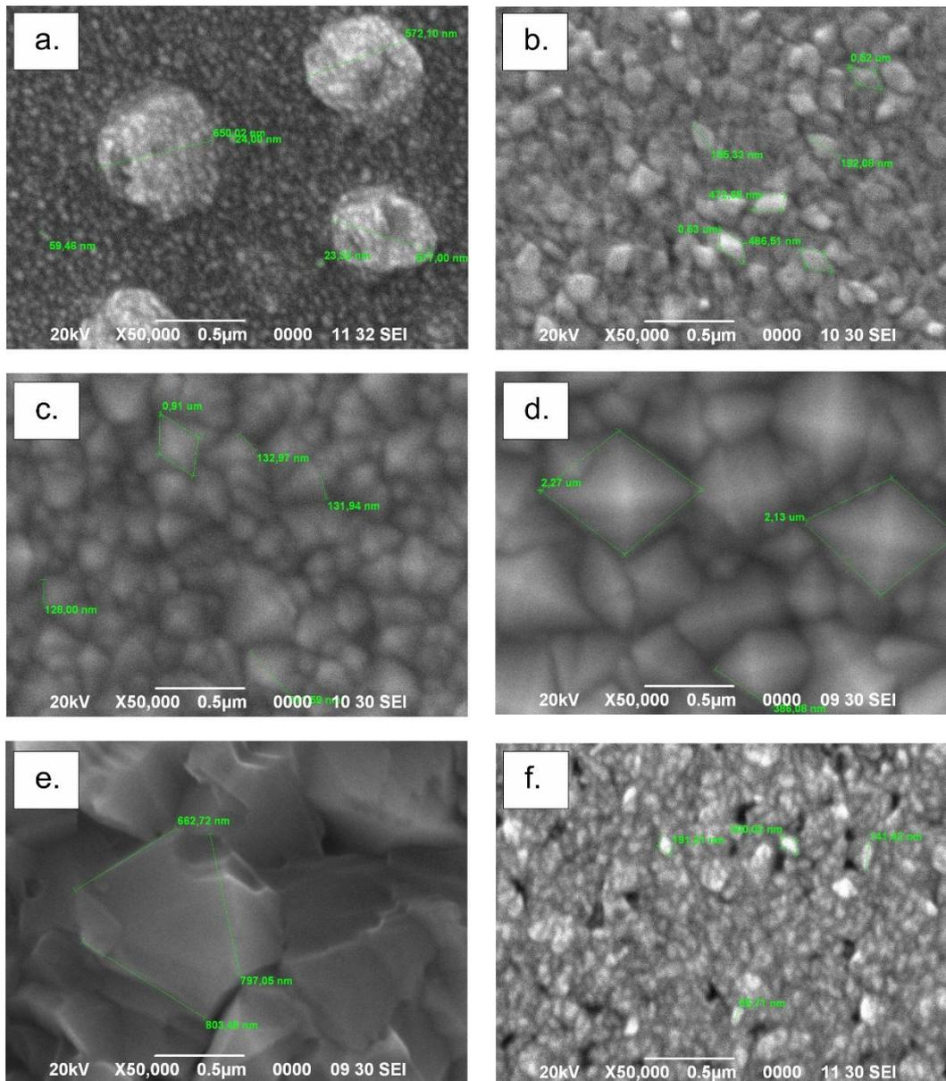
Figure 8 SEM microstructure of FTO thin film on 50,000 $\times$  magnification: (a) 2%-300-5'; (b) 2%-300-10'; (c) 2%-300-20'; (d) 2%-300-30'; (e) 2%-300-40'; (f) 0%-300-20'
