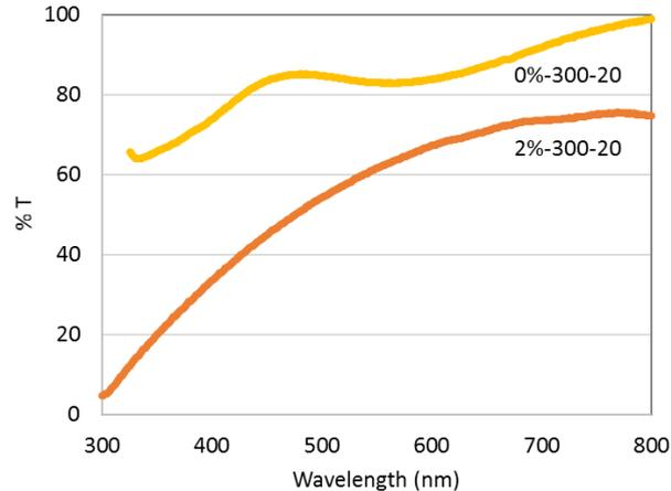
Figure 6 Transmittance Vs wavelength in undoped (0%-300-20') and doped (2%-300-20') samples
