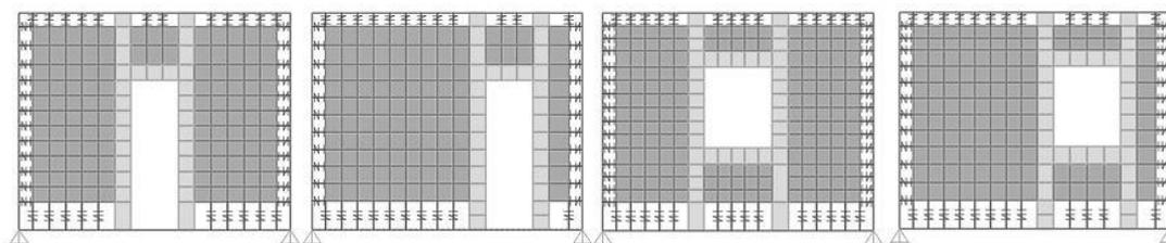
Figure 1 IFcO models with cantic and eccentric door and window openings
