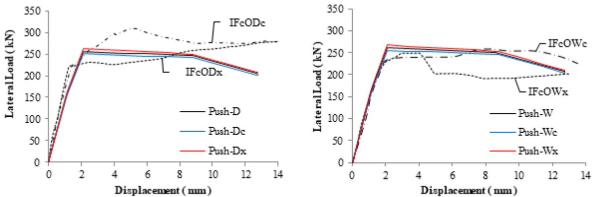
Figure 3 Pushover curve of IF with door and window (right) openings compared to previous test results
