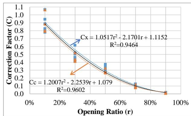
Figure 2 Correction factor associated with opening ratio
