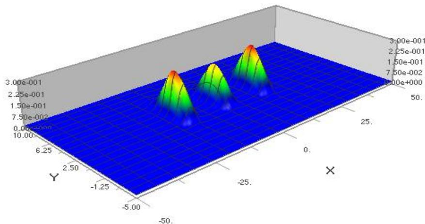
Figure 4 Optical intensity field distribution at the splitter output
