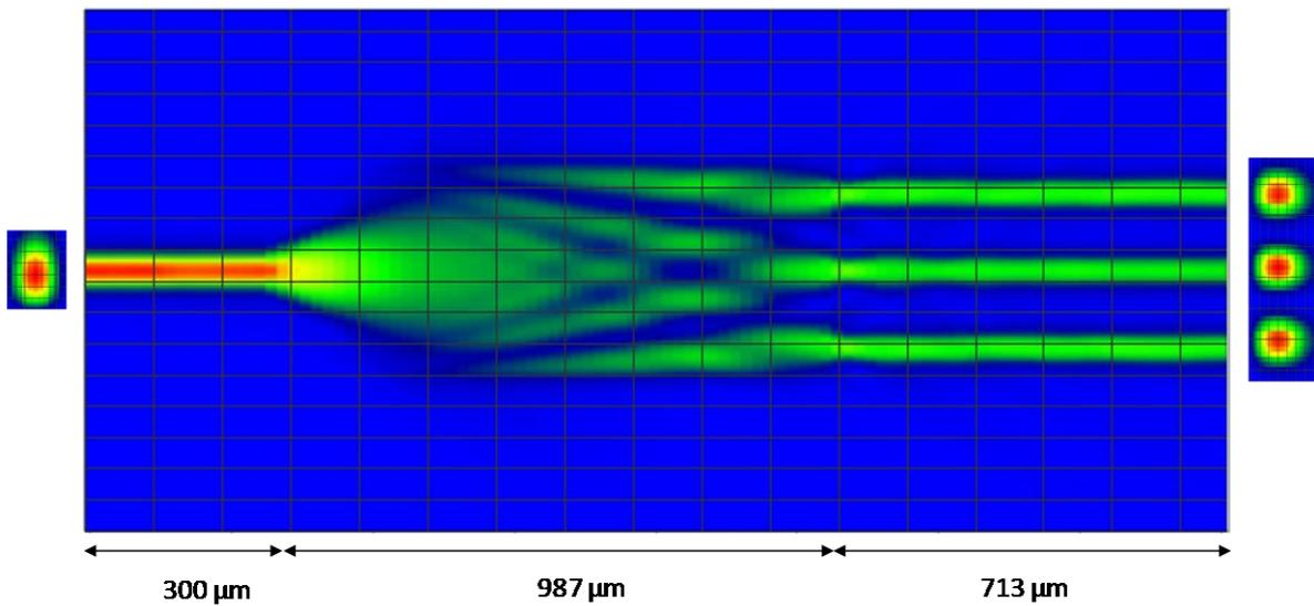
Figure 3 Optical intensity field distribution of the proposed 1×3 Power Splitter, when total length  $L=2000 \mu\text{m}$  and  $W_{MMI} W=40 \mu\text{m}$
