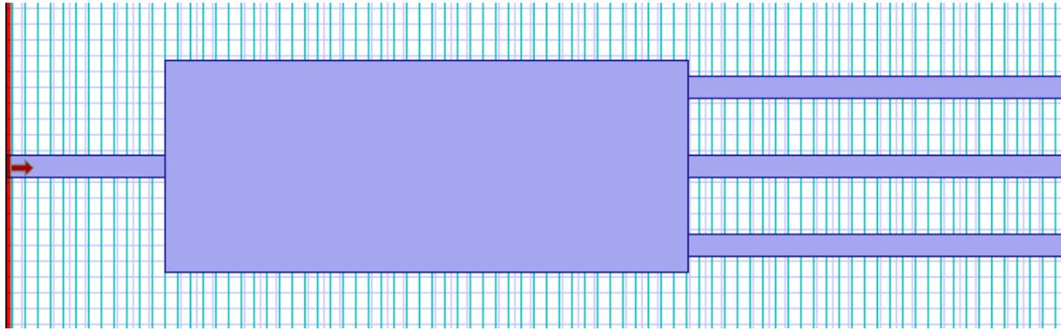
Figure 2b The proposed 1×3 optical power splitter
