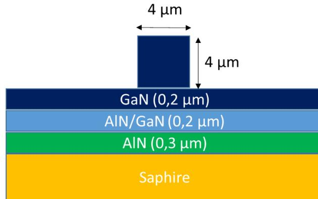
Figure 2a Cross section of input power splitter
