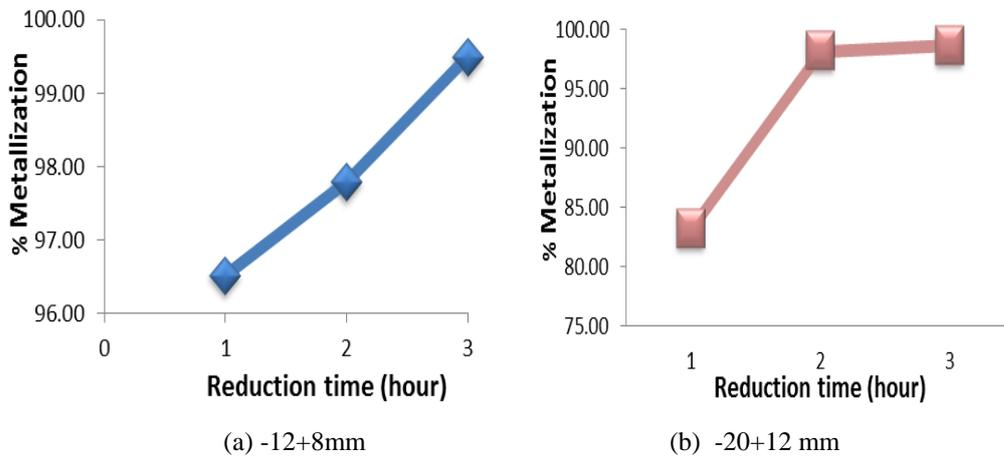
Figure 4 Effect of reduction time on a percentage of metallization of sponge iron
