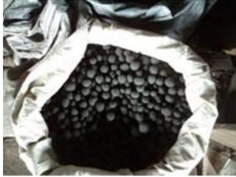
Figure 1 South Lampung iron ore pellets, which are mixed with coconut shell charcoal and bentonite
