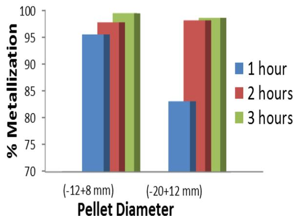
Figure 5 Effect of pellet diameter on a percentage of metallization of sponge iron
