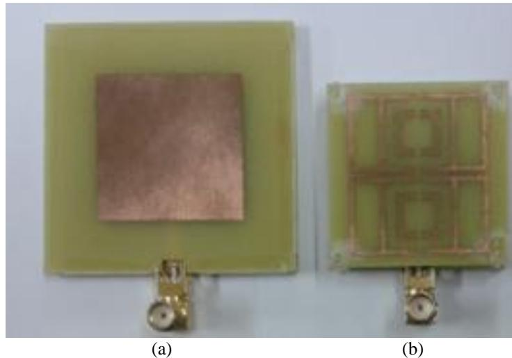
Figure 8 Photograph of microstrip antenna: (a) without LHM; and (b) with LHM structure
