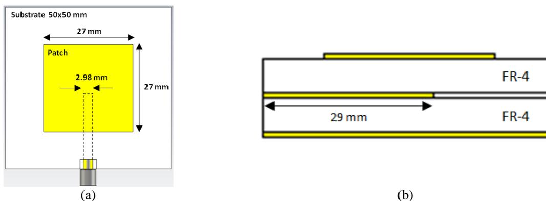
Figure 1 Geometry of conventional antenna design (a) Top view (b) Side view
