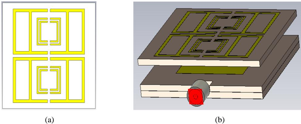
Figure 6 (a) Design of LHM structure for gain enhancement; (b) Exploded view of single element antenna with LHM structure on top
