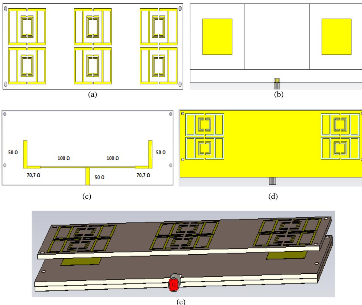
Figure 9 Design of two element array LHM antenna: (a) Gain enhancement element; (b) two element patch antenna; (c) Power divider; (d) bottom view of antenna; (e) exploded view of antenna
