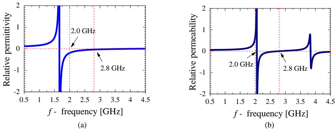
Figure 5 Single cell LHM: (a) negative permittivity; (b) negative permeability
