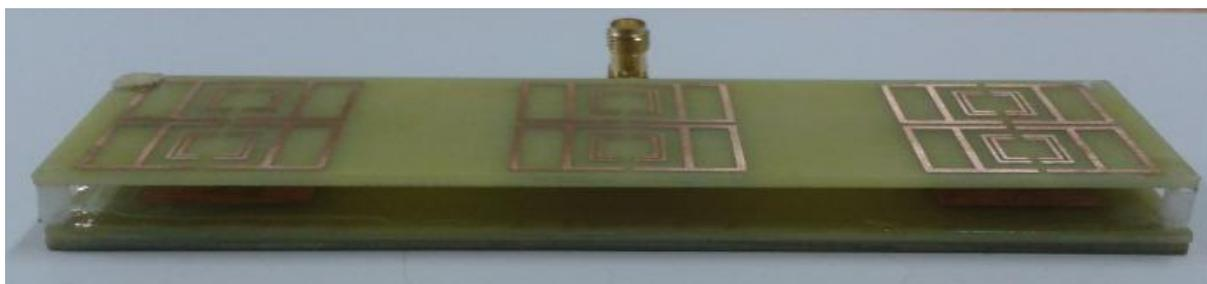
Figure 10 Photo of two-element microstrip antennas array with LHM
