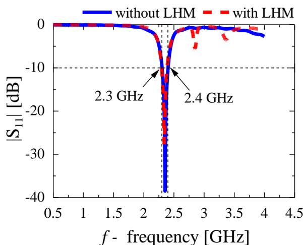
Figure 7 Simulation result of reflection coefficient antenna with and without LHM structure
