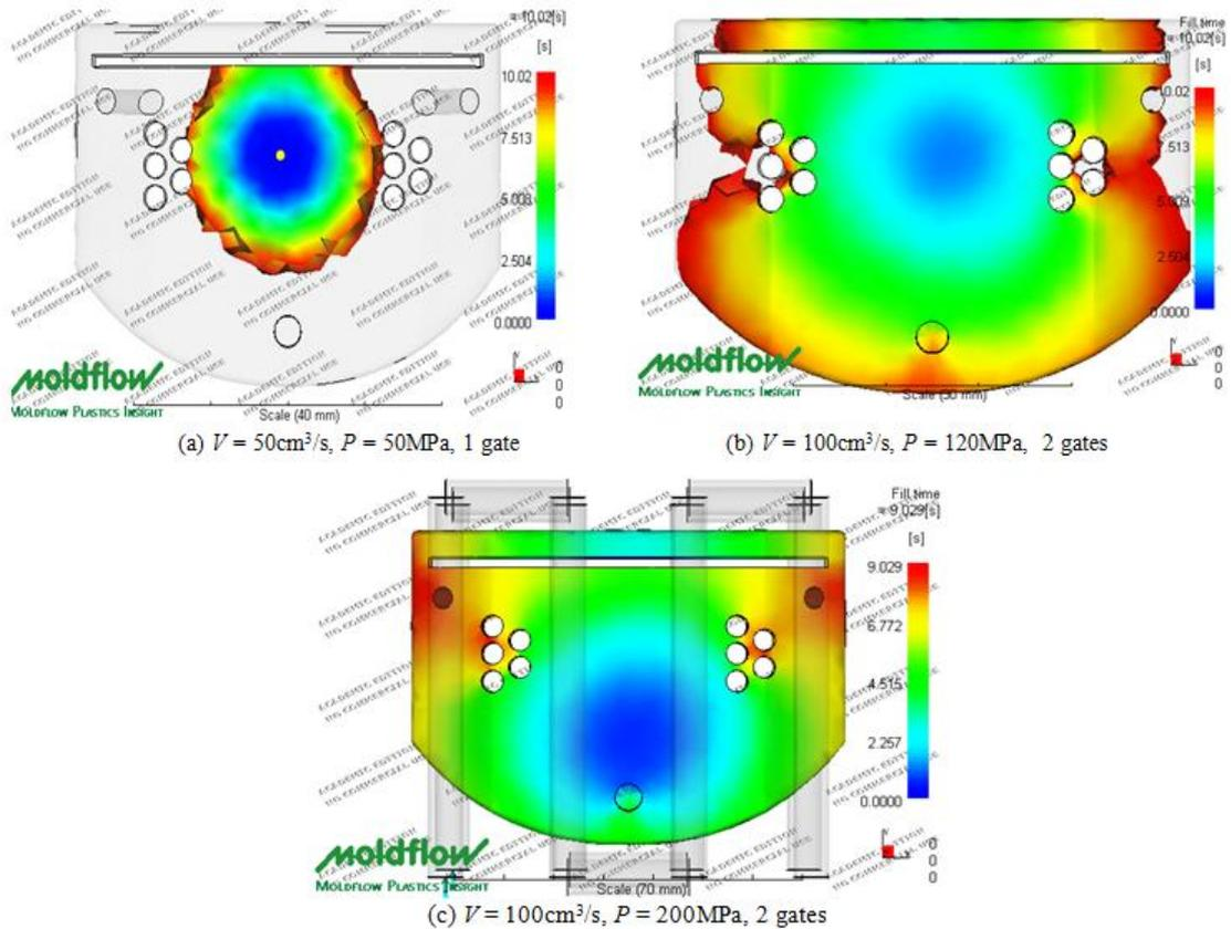
Figure 8 Simulated filling of the jig pattern under various conditions
