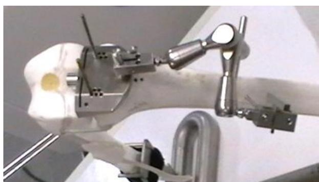
Figure 6 Locating the prototype jig on sawbone cutting
