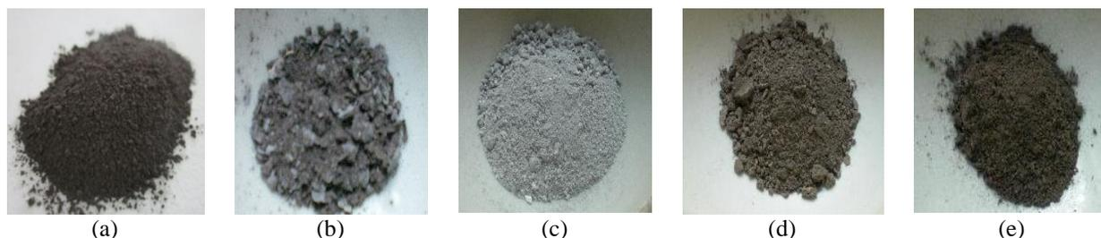
Figure 3 Physical appearance of the results after magnesiothermic reduction at: (a) 750°C for 2 h; (b) 800°C for 3 h; (c) 850°C for 3 h; (d) 900°C for 3 h; (e) 950°C for 3 h
