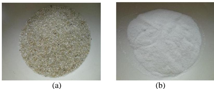
Figure 1 Quartz sands from Tanjung Tiram, Asahan: (a) prior to separation; (b) after separation
