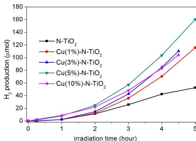
Figure 6 Effect of Cu dopant on the performance of TiO<sub>2</sub> in producing hydrogen from glycerol and water (10 % v/v glycerol) over various irradiation time intervals
