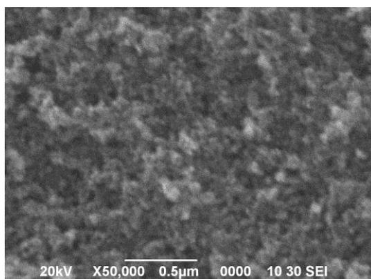
Figure 3 SEM topography of Pt(1%)-N-TiO<sub>2</sub>
