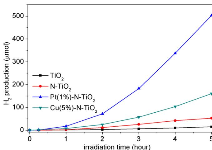
Figure 7 Effect of N, Pt and Cu dopant on the performance of TiO<sub>2</sub> in hydrogen production from glycerol and water (10% v/v glycerol) over various irradiation time intervals
