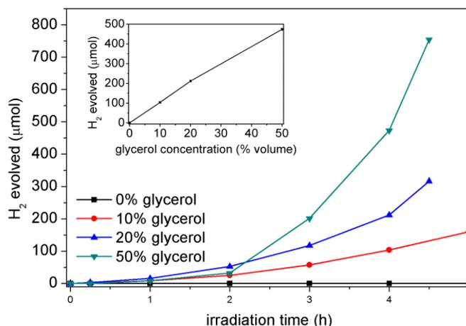
Figure 8 Effect of glycerol concentration on hydrogen production (photocatalyst: 500 mg of Cu(5%)-N-TiO<sub>2</sub>) over various irradiation time intervals
