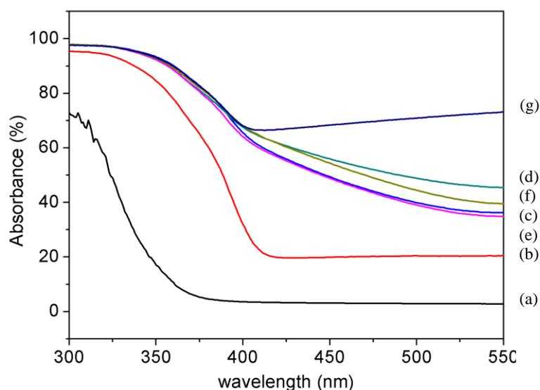
Figure 1 DRS spectra of: (a) TiO<sub>2</sub>; (b) N-TiO<sub>2</sub>; (c) Cu(1%)-N-TiO<sub>2</sub>; (d) Cu(3%)-N-TiO<sub>2</sub>; (e) Cu(5%)-N-TiO<sub>2</sub>; (f) Cu(10%)-N-TiO<sub>2</sub>; (g) Pt(1%)-N-TiO<sub>2</sub>
