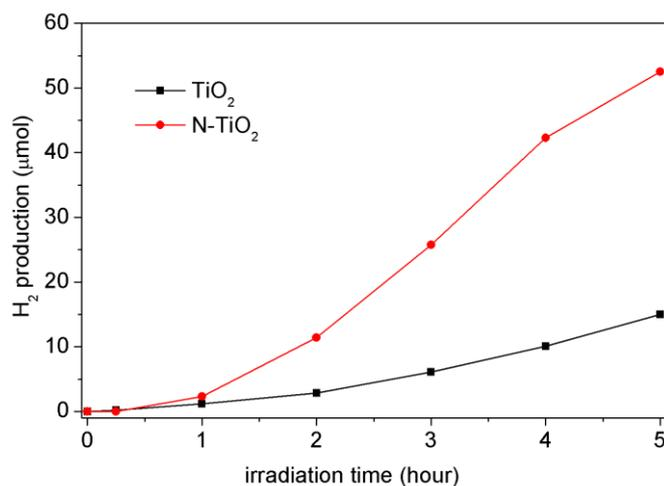
Figure 5 Effect of nitrogen addition on the hydrogen production from glycerol and water (10 % v/v glycerol) with various irradiation time
