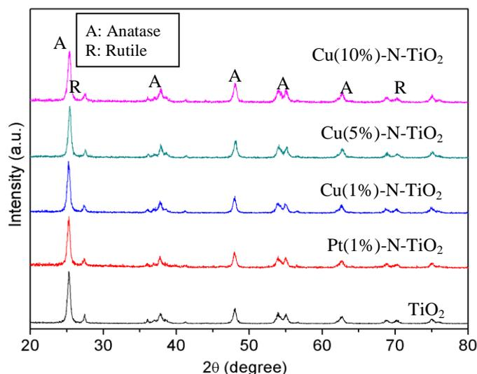
Figure 2 XRD diffraction patterns of  $\text{TiO}_2$ , Pt-N- $\text{TiO}_2$  and Cu-N- $\text{TiO}_2$
