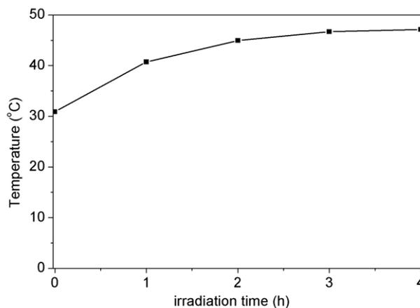
Figure 9 Effect of irradiation time to the temperature profile of the reaction system
