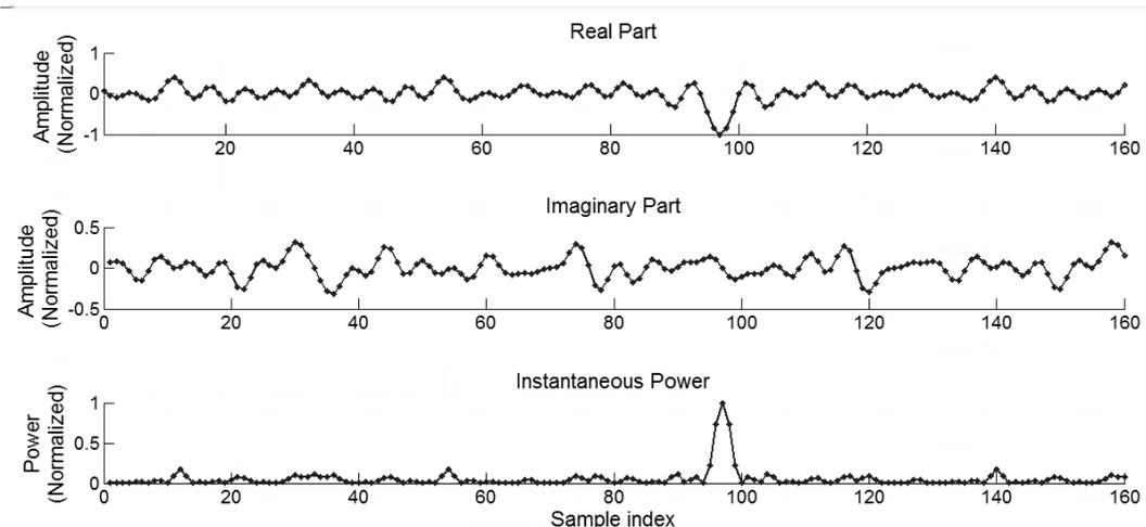
Figure 6 L-SIG signal that has maximum PAPR
