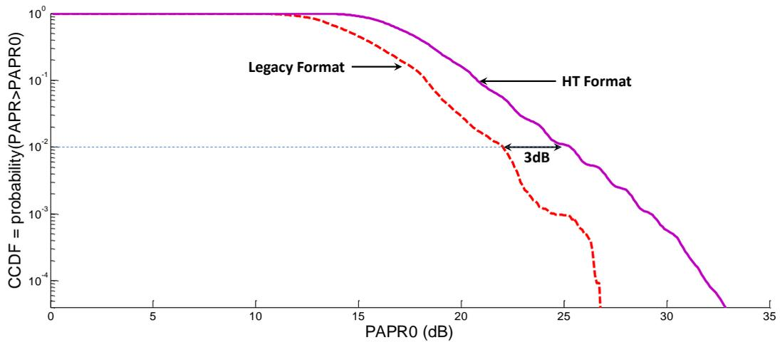
Figure 11 CCDF for Legacy format and HT-format
