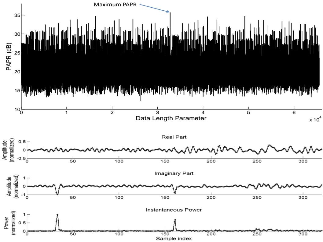
Figure 8 HT-SIG signal that has maximum PAPR
