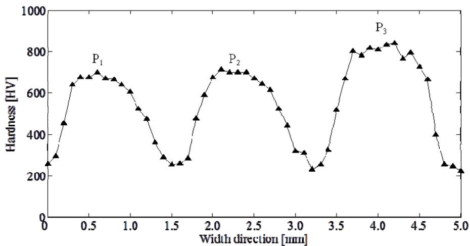
Figure 4 Hardness profile of non-overlapping scans
