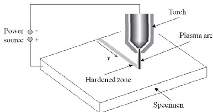
Figure 1 Schematic diagram of experimental setup
