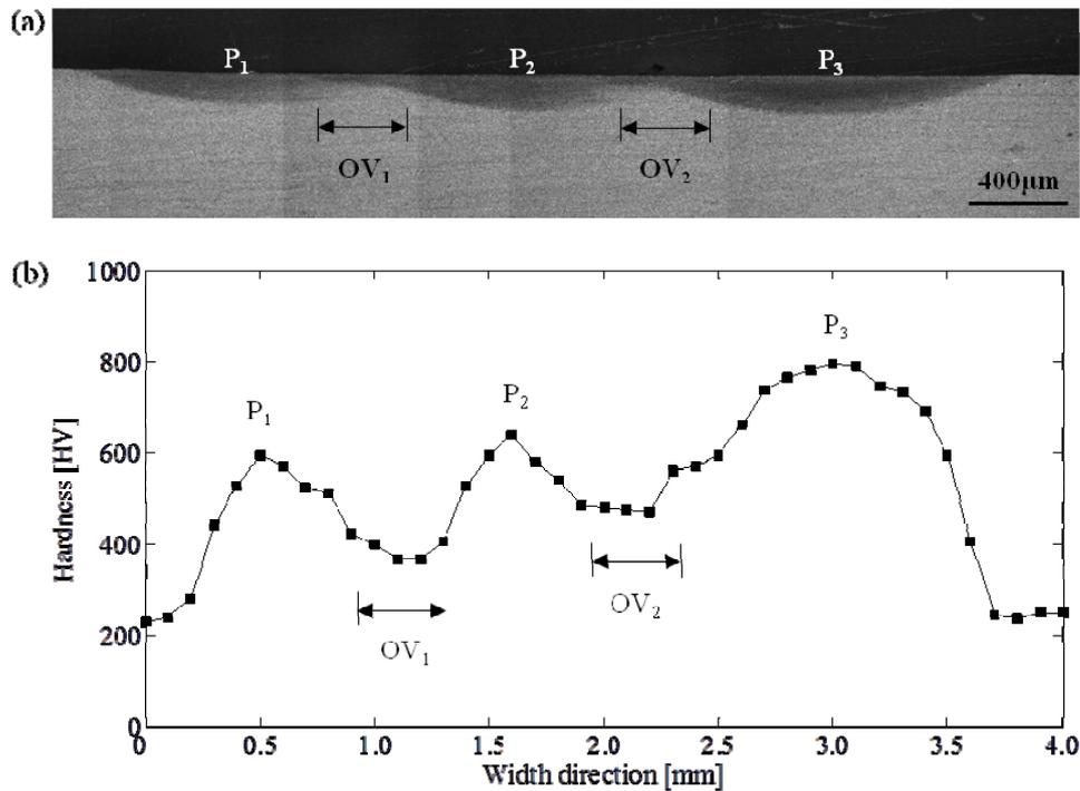
Figure 3 (a) Optical micrograph of the cross-section of the hardened specimen with overlapping scans; (b) microhardness measurements along the subsurface at a constant depth of 30 μm and perpendicular to the plasma arc passes direction
