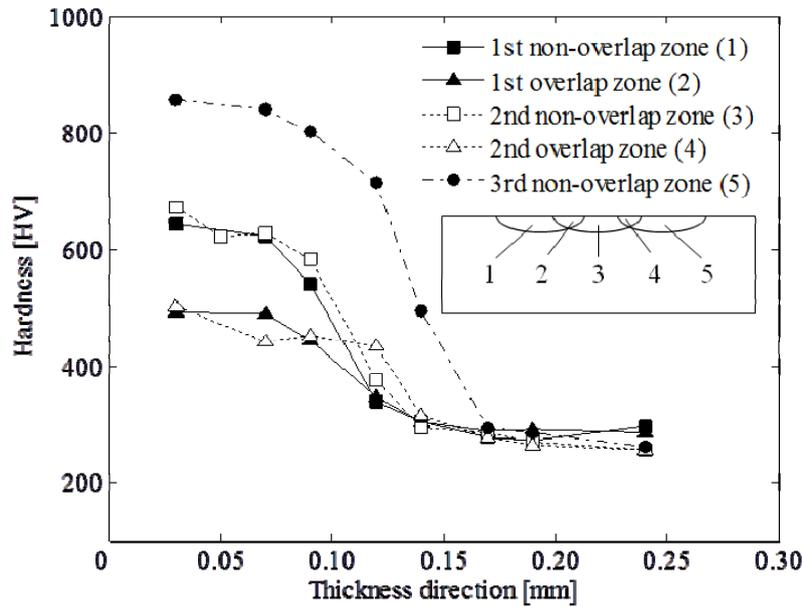
Figure 5 Hardness profile of plasma arc hardened in multiple passes
