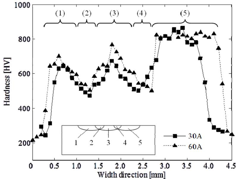
Figure 7 Hardness distribution of multiple passes with different arc currents
