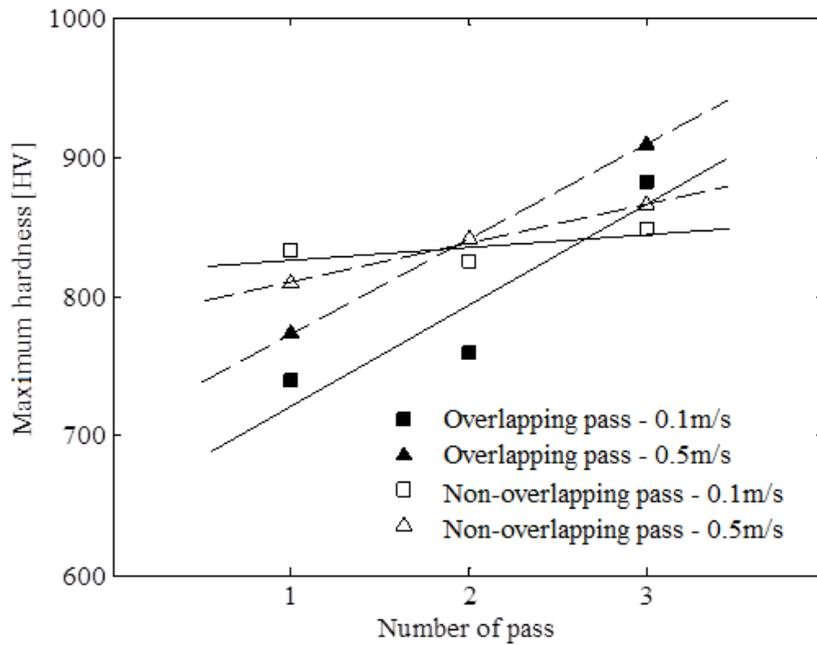
Figure 9 Maximum hardness of multiple passes versus number of plasma arc scan
