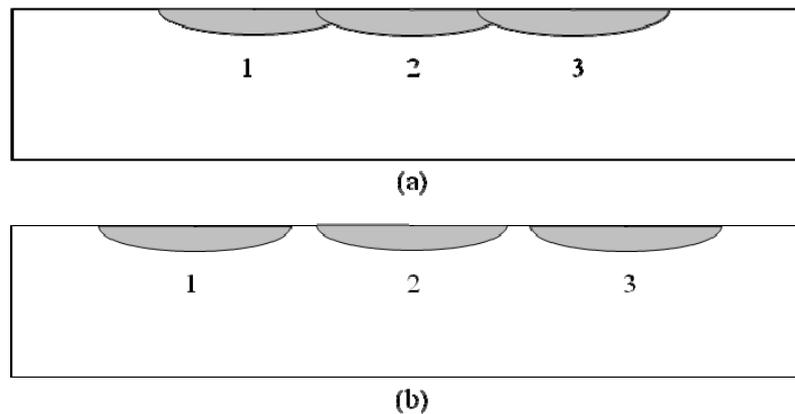
Figure 2 Schematic diagram of multiple passes in cross-sectional view (a) with overlapping scan of 20% and (b) without overlapping scan
