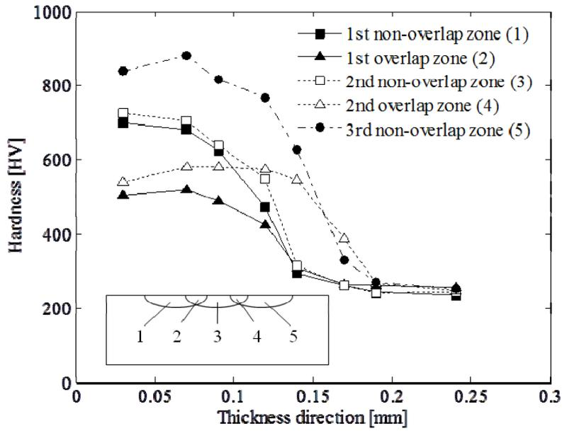
Figure 8 Hardness profile of plasma arc hardened with high 60 A arc currents
