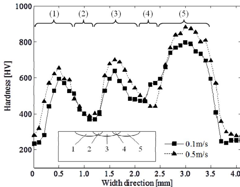
Figure 6 Hardness distribution of multiple passes with different scanning velocities
