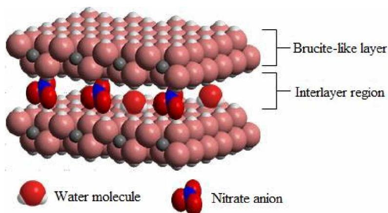
Figure 1 Schematic diagram of LDH structure with nitrate as the interlayer
