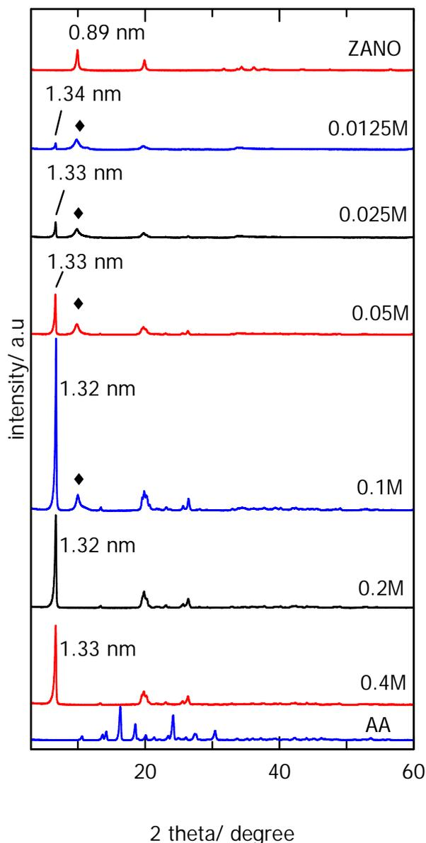
Figure 3 XRD patterns for ZANO and ZAAN at different concentrations of AA
