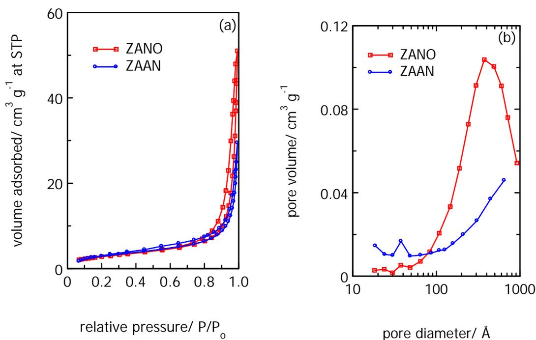
Figure 5 (a) Adsorption-desorption isotherms and (b) BJH pore size distribution for ZANO and ZAAN
