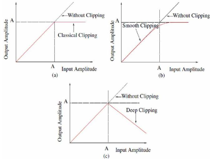
Figure 1 Clipping transfer functions: (a) classical clipping, (b) deep clipping, (c) smooth clipping (Guel & Palicot, 2009)
