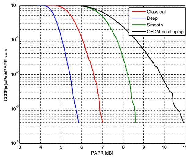
Figure 4 CCDF comparison, system without LDPC codes
