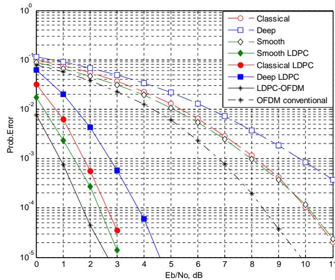
Figure 6 BER performance for CC, DC, and SC with and without LDPC
