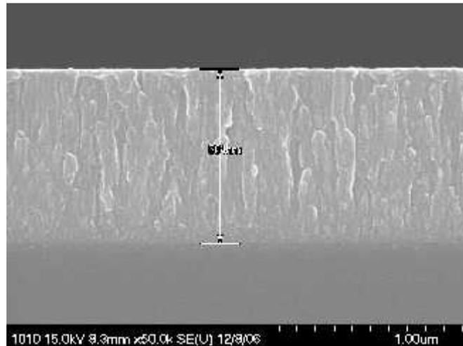
Figure 1 Ti-10Ta-10Nb thin film with the thickness of 964 nm deposited on CP Ti substrate by dc magnetron sputtering
