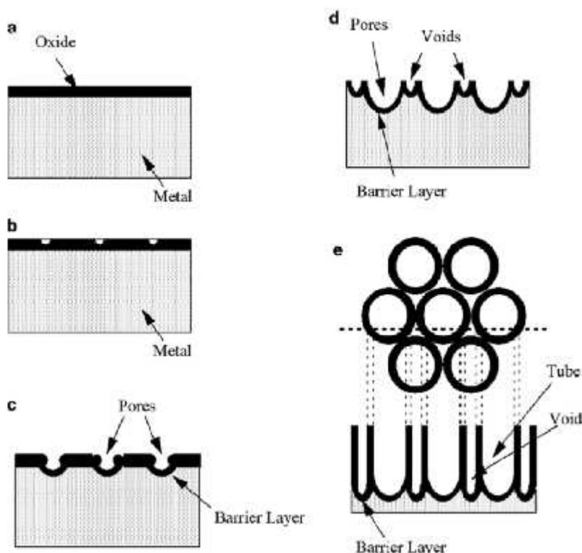
Figure 4 Schematic diagram of nanotube evolution at constant anodization voltage: (a) Oxide layer formation, (b) Pit formation on the oxide layer, (c) Growth of the pit into scallop shaped pores, (d) The metallic region between the pores undergoes oxidation and field assisted dissolution, (e) fully developed nanotubes with a corresponding top view (Mor et al., 2003).
