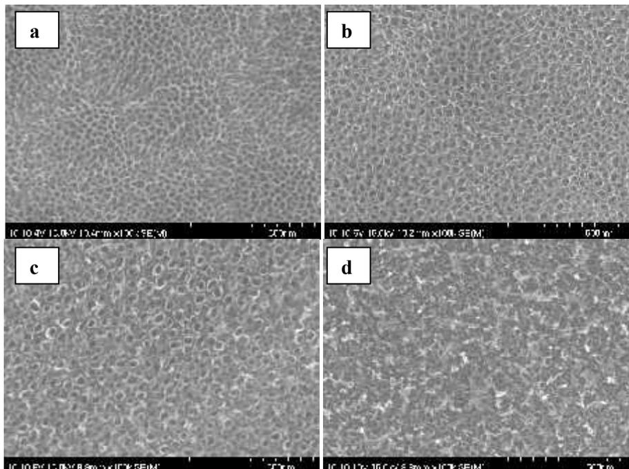
Figure 2 Size of nanotubes on Ti-10Ta-10Nb thin film by anodization in the solution containing 1M H<sub>3</sub>PO<sub>4</sub> + 1.5wt.% HF at the applied potential of (a) 4 V, (b) 6 V, (c) 8 V and (d) 10 V
